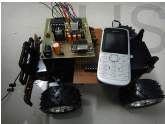
Fig. 4 Top view of mobile phone controlled autonomous robot
